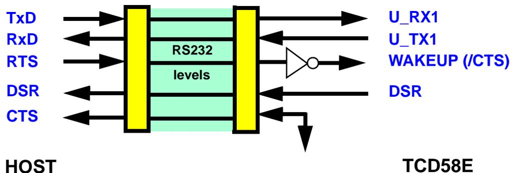
1. The support by the TCD58E of Host DSR and RTS signals is not completely standard: they are used for an advanced system wake-up implementation. Please contact AuthenTec for further details. Please note the inversion of the RTS/CTS signal.
