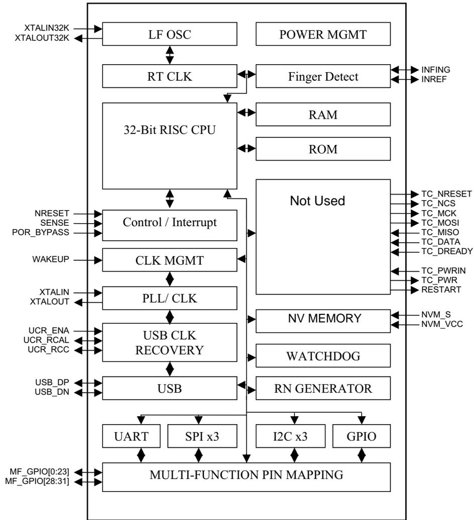
Note that the SPIX interface is not used in this implementation. The sensor data buss and control lines are primarily sourced from the multi-function pins. See the appropriate reference design for details.
