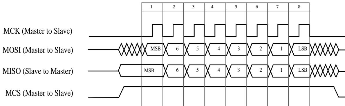
Note: MCS shown terminating after one byte for illustrative purposes only, actual transfers must maintain MCS in the active state for one frame of 9 bytes.
